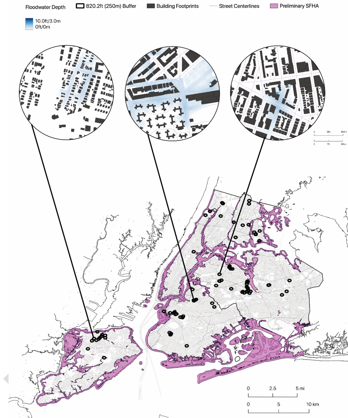
Figure 7: 83 high water marks (HWM) such as seed lines, mud, and debris were surveyed by the US Geological Survey in the weeks following the Ida-Remnants Cloudburst (Finkelstein et al., 2023). Using these observations, land surface inundation was estimated within an 820.2 ft (250m) buffer of each observed HWMs. During the Ida cloudburst, deep inundation from pluvial flooding occurred in areas that were far from the water bodies used as the basis of FEMA SFHA modeling. Flooding from this event was not limited to areas where HWMs were obtained and occurred in areas of the city that were not surveyed or where HWMs could not be identified. Several inundated areas are highlighted here and all HWM data from this survey can be viewed at: https://stn.wim.usgs.gov/fev/#2021Ida . Map by BR Rosenzweig.
